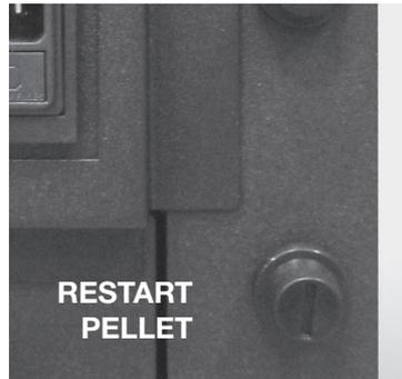
**Pellets temperature safety:** In the rare event there is a too high temperature in the tank, the thermostat for pellets safety with manual reset creates an alarm **"ALAR-SIC-FAIL"** stopping the pellet boiler stove. You need to reset the system working on the device placed on the back of the stove.
