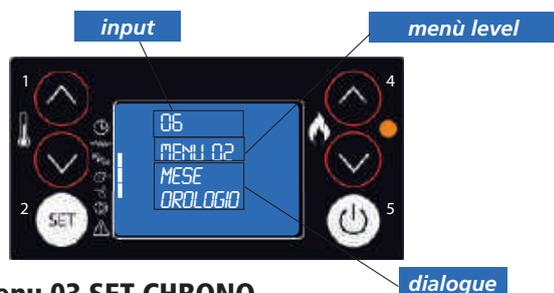
Set the current time and date. The device comes equipped with a lithium battery that allows the internal clock to operate autonomously for over 3-5 years.
