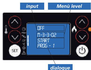
The weekly programmer has 4 independent programmes whose final effect is composed of the combination of the 4 individual programmes. The weekly programmer can be activated or deactivated. Additionally, by setting OFF in the time field, the clock ignores the corresponding command.
