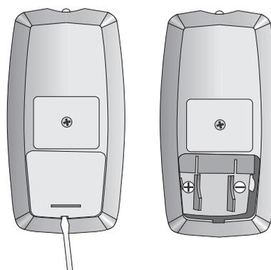
Pict. 22: Replacing batteries in the remote control (if supplied)
