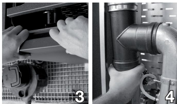
Raise the stove front to release the "T" fitting containing compartment. (foto 3)
