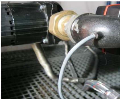
Temperature probe for auxiliary heating systems (puffer or accumulators)
